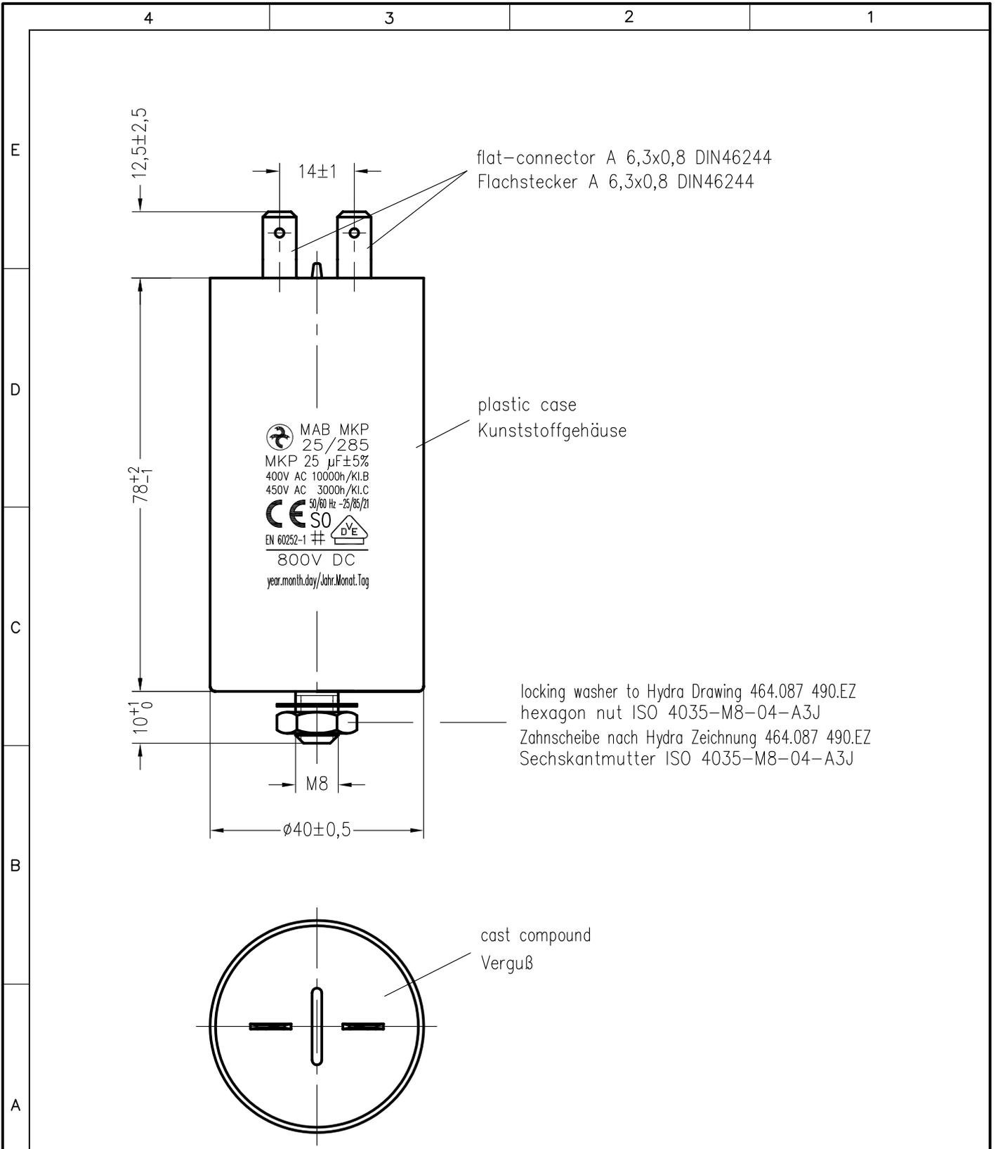
flat-connector A 6,3x0,8 DIN46244
